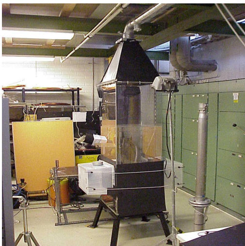
Figure 11. General view of secondary air jets visualisation model at TUT on left (a), view of secondary air jets behaviour and measuring of penetration with rod in a certain test (b).
