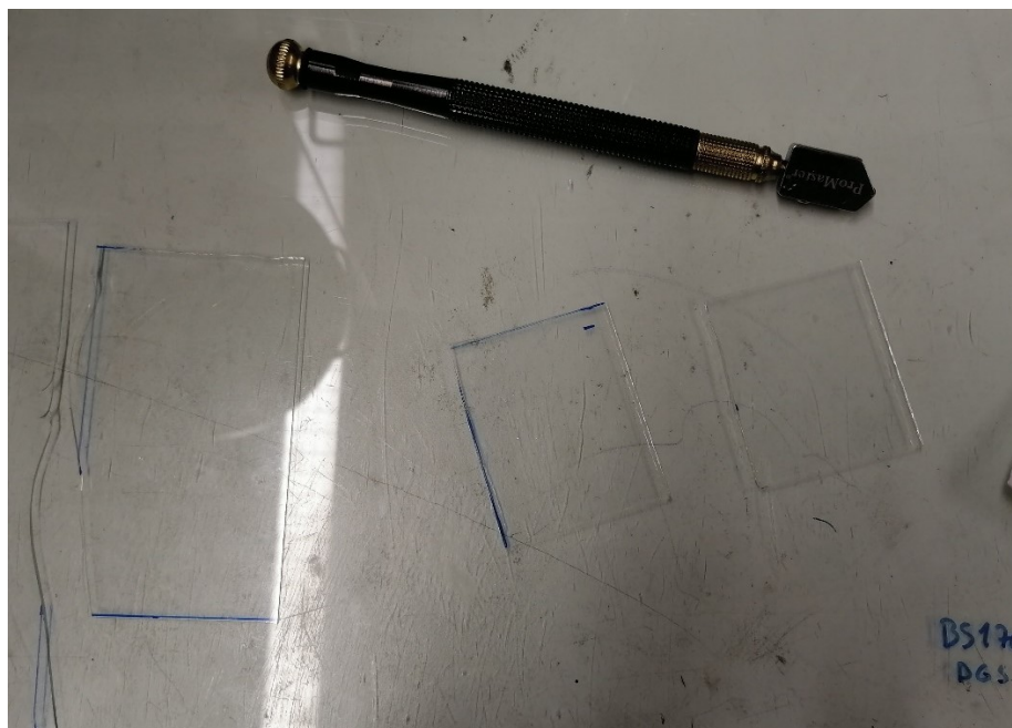
Image 2.2. The reflection glasses cut from the bigger glass plane.
