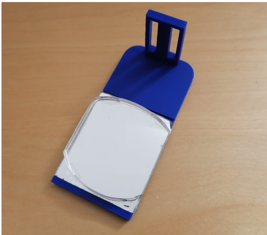
Image 2.9. The lens-mirror package on the lens-mirror-holder.
