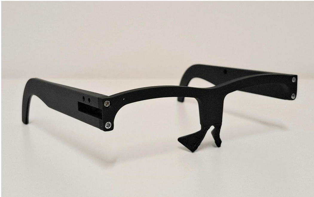
Figure 4.1. OpenAR-M frame and temples. The frame has a tunnel for hiding electrical wires.
