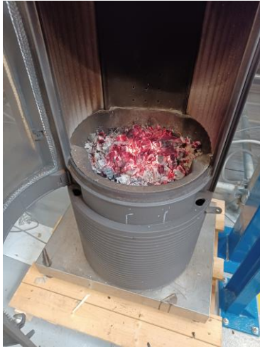
1. Initial phase (Preheating) No flame, \text{CO}_2 < 4\% Ember bed \sim 3 \text{ cm}
