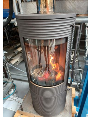
3. Combustion tests Start: straight after wood load (door closure) End: No flame, \text{CO}_2 < 4\%
